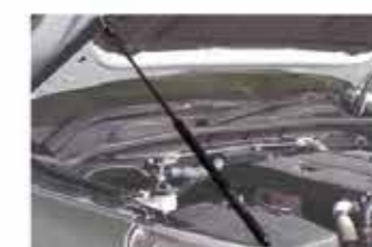
CB-548 Hood Lifter Designed for your convenience to lift and hold the hood.
