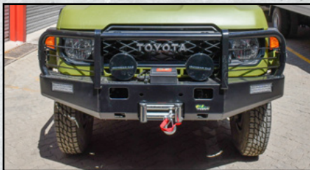
Winch-compatible bull bar with jacking slots
