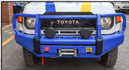
Winch-compatible bull bar with jacking slots
