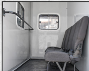
Bench seat with 2-point safety belts
