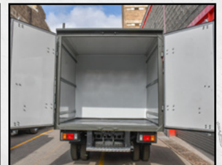
Dry-cargo compartment with side cargo rails
