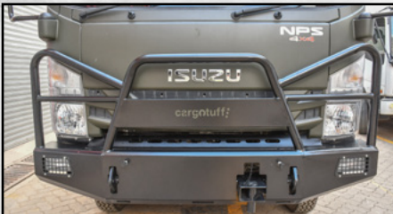
Bullbar with integrated fog lamps and heavy duty tow-hook
