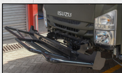
Forward tilting bullbar for engine bay access
