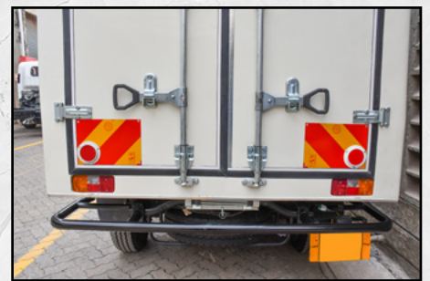
Double-lip, waterproof lightweight rear doors
