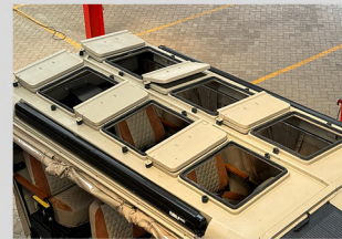
Fibreglass Roof w.Hatch
